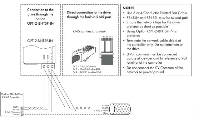
Modbus RTU and BACnet MSTP connection should be made via the RJ45 connector. The pin assignments are as shown in section 11.1. RS-485 communications.
