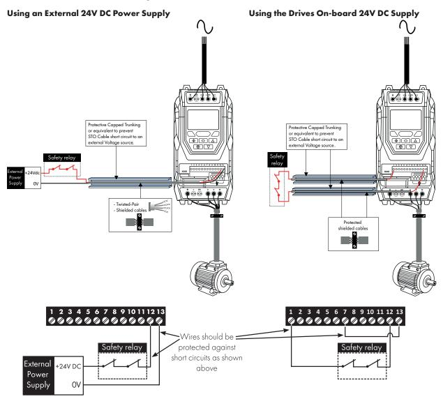
NOTE The Maximum cable length from Voltage source to the drive terminals should not exceed 25 metres.
