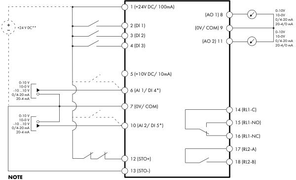
\* Dashed lines shows connection for analog inputs in digital mode \*\* Optional external 24 V DC power supply
