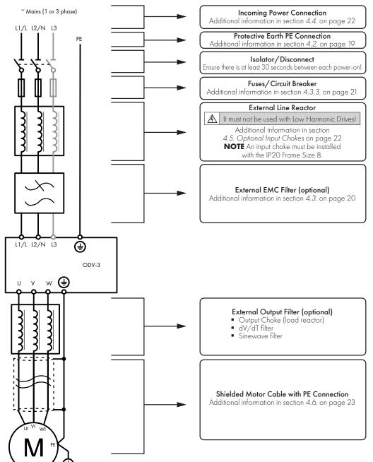
NOTE Enclosed drives are not suitable for rigid conduit system connection.
