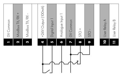
STO signal must be provided in order to permit running the motor. Start/Stop command provided by the Digital Input. The speed reference is provided by the output of the PI controller and the PI feedback is provided by the analogue input.
